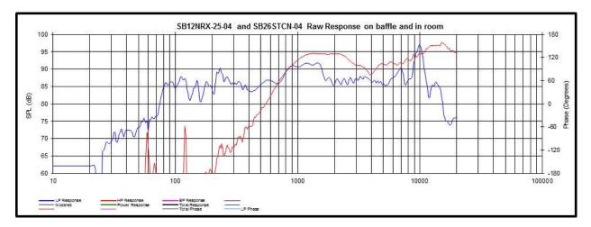
Here's the raw response at one meter on the baffle - no fancy smoothing here.
