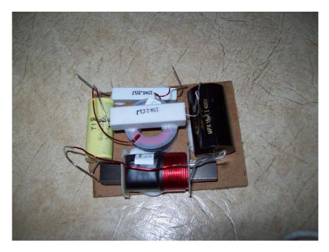
Make sure your crossover boards can fit through a hole 3.75" in diameter. Here's how I laid mine out on the board.
