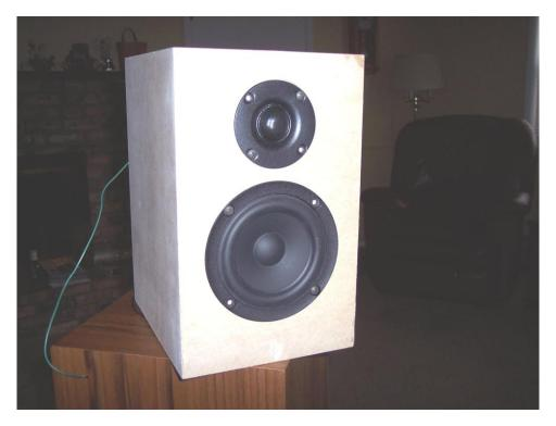
These speakers are ported on the back. I used a standard 1.25" diameter adjustable port that Meniscus sell. To make it even easier, I used only the inside section with the mounting flange. This leaves the port a little over 4" long and tunes this enclosure to 61Hz. However, since this port is adjustable I will give you some options. Here's a pic of the front and back of the finished painted enclosure.
