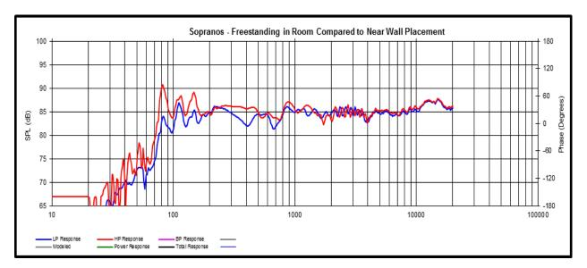
The effect of the boundary can be seen, but the design works well in either location. The dip in the response in the free-field response is similar to that of the LS3/5a and is not nearly as noticeable as you might be inclined to think, and vocals sound extremely lifelike and open from these speakers. These Sopranos really sing.
