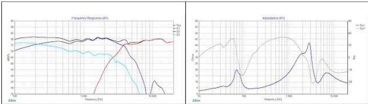
The impedance load of this design would probably be considered 4 Ohms nominal, however it just barely dips down there, and on the whole should be pretty benign for most solid state amps and home theater receivers. It's no worse than the OSMTM.
